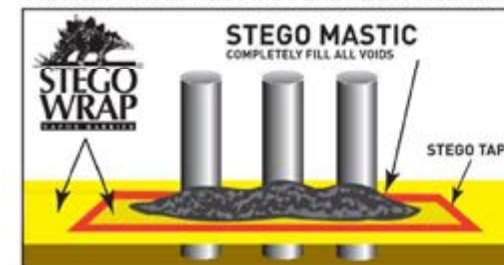
FIGURE 5: MULTIPLE PIPE PENETRATION SEALING
