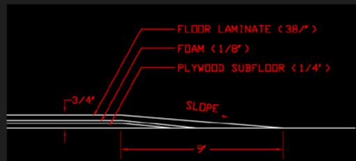
It is a code requirement to comply with the ADA. (1"=12" TRANSITIONAL SLOPE).
