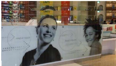
Graphics must be mounted behind frameless glass or acrylic. An option is to mount the graphic behind glass/acrylic on stand offs.
